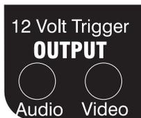
The other two trigger outputs carry one signal each. The Main Trigger connection has 12 volts DC when the Maestro is turned on. The Video Trigger jack goes to 12 volts when one of the video sources is selected.
