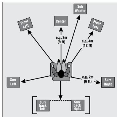
It is critical to properly match the levels from each speaker to achieve a correct sound stage. The realism is totally lost if the footprints of a person walking across the screen change in volume as they move from left to center to right. We strongly recommend using a test analyzer such as our Iasys HT for this calibration. The levels are nearly impossible to judge by ear alone. Though not as accurate as using the Iasys HT, you can use a sound level meter for this adjustment.
