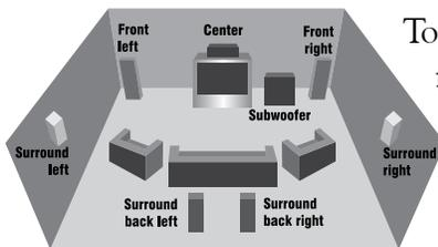
To present the most realistic sound stage, all three of the front speakers must be tonally balanced. Ideally, these speakers should be identical models. This ensures that the sound doesn't change as it pans across the screen. Place the speakers at the seated ear level. Whenever possible, the three front speakers should also be placed at the same horizontal level for best imaging.
