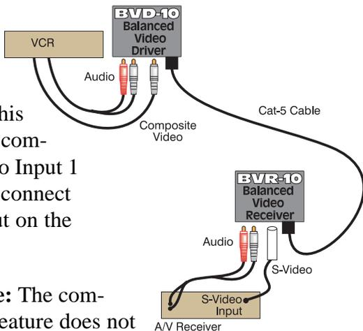
**Installation Note:** The composite to S-Video feature does not function on Video Input #2.
