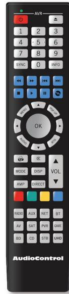
The supplied remote control is an eight device “universal” IR remote controller with back-lit gum-drop buttons. Use the remote for full control of the Processor/Receiver, plus various AV sources and displays via the extensive library of device codes. A complete list of codes is available on our Knowledge Base at: [audiocontrol.com/knowledge-base/](http://audiocontrol.com/knowledge-base/). Search "program htr-3".
