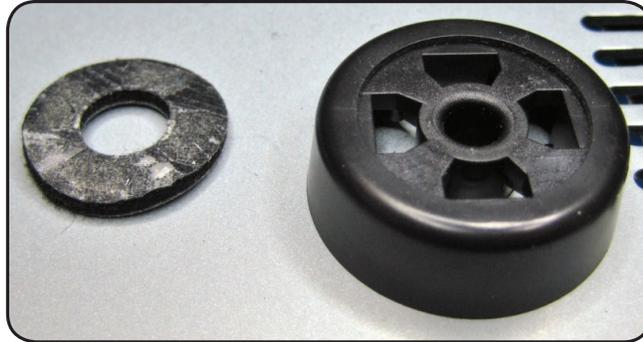
4. Identify the four locking tabs securing the foot to the chassis. The photo of a removed foot shows the details of the locking tabs.
