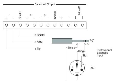
You can use the Balanced Line Series components to convert from -10dB unbalanced RCA to a balanced signal to drive professional audio equipment. Make certain that you set the gain controls per the chart on the previous page to bring the signal level up to pro specs.
