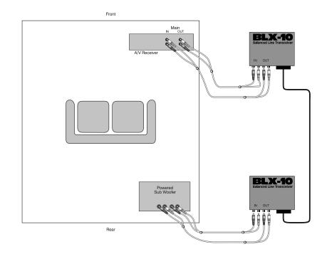
The Balanced Line Series provides a noise-free method to extend the distance between components in an audio system. This allows you to put the amplifiers in the Basement and the source units in the Library or put a CD player in the Master Bedroom and run the audio to your Media Room. They are also handy if a powered subwoofer is picking up noise from a long RCA cable run from the surround processor.
