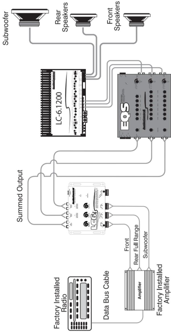
**Figure 6:** Six channel system with LC6i and EQS
