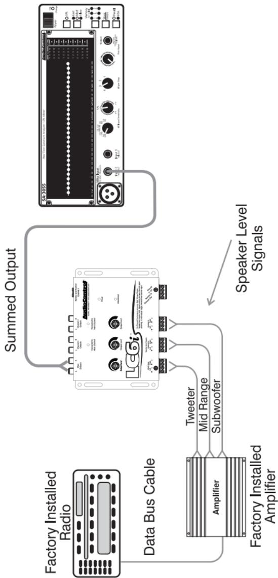
**Figure 7:** Using an RTA to measure the Summed Response
