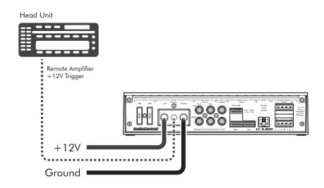
In this example, the head unit has a +12V trigger output that is connected to the LC-4.800's remote input terminal. When the head unit is turned on, it will turn on the LC-4.800 amplifier.
