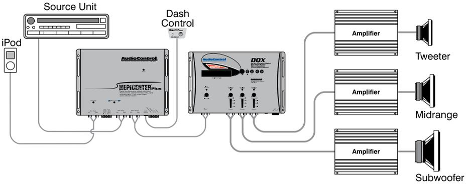
Figure 5: Two channel system with equalizer and crossover
