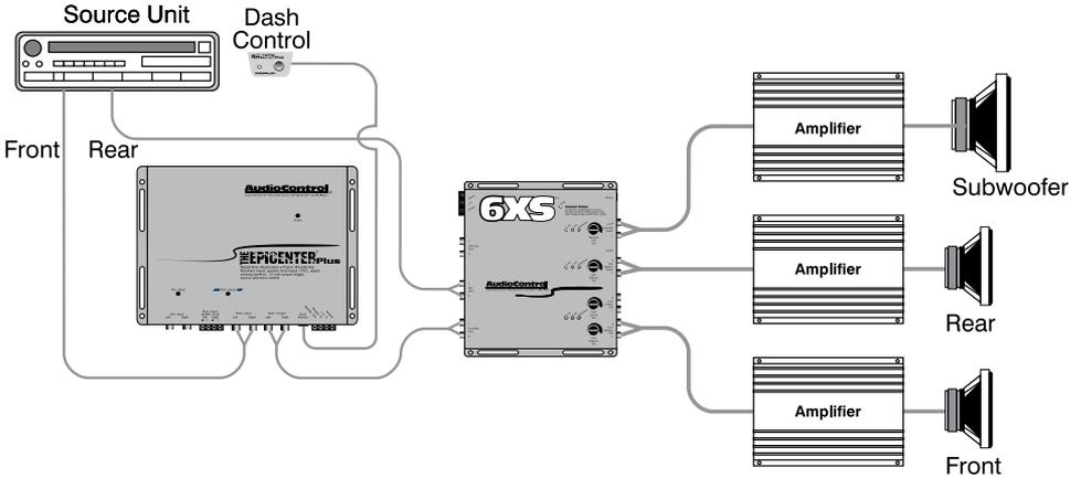
Figure 6: Four channel system with crossover
