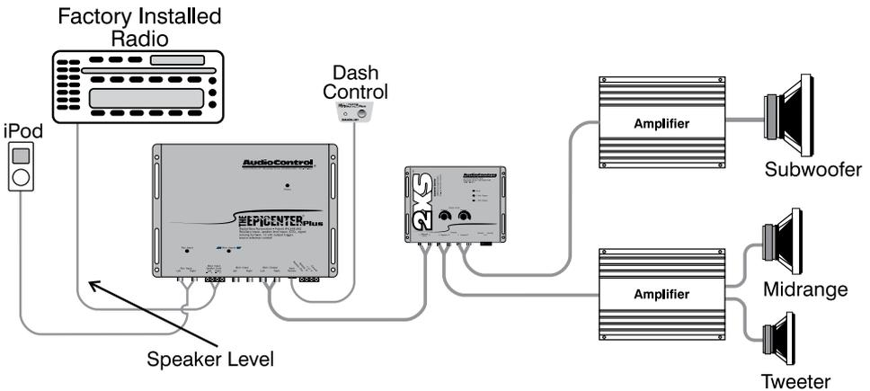
Figure 1: Basic Installation Of The Epicenter Plus
