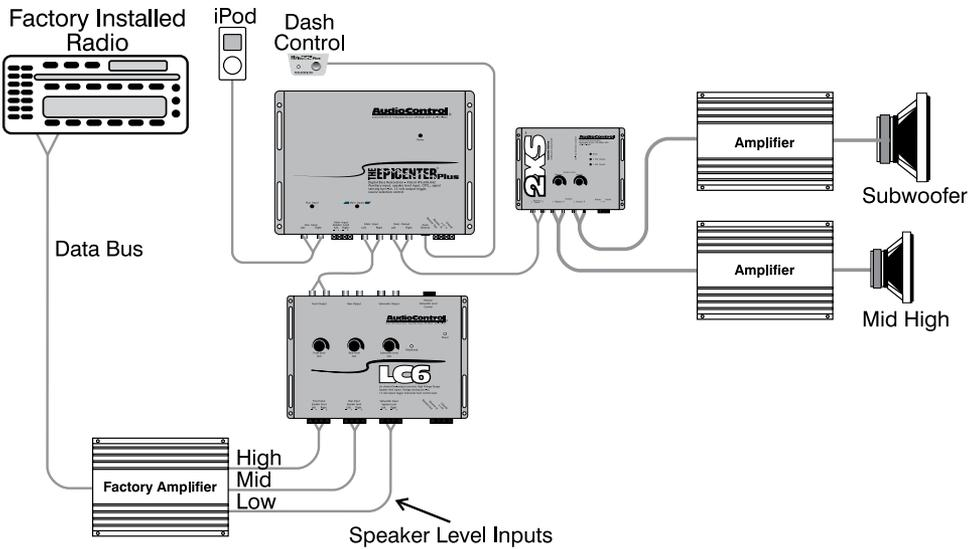
Figure 8: Interfacing with a factory installed radio/amplifier using an AudioControl L6i for signal summing
