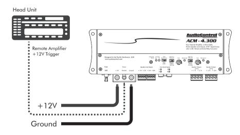
In this example, the head unit has a +12V trigger output that is connected to the ACM-4.300 remote input terminal. When the head unit is turned on, it will turn on the ACM-4.300 amplifier.
