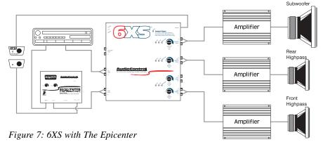
**AutoMode Inputs:** If your source unit has front, rear, and subwoofer outputs (aka "six channel"), connect them to the identical inputs on your 6XS. However, if you are only using front and rear signals (four channel) or just two channels, the Auto Mode circuitry in your 6XS will automatically feed your subwoofer channel with signal from your front inputs.
