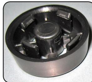
5. Use the small flat-bladed screwdriver to gently pry the four locking tabs outward to release the foot from the chassis. Use the needle-nose pliers to pull upward at the same time, with (to get all technical for a moment) a bit of a jiggle-joggle motion.
