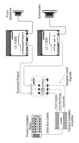
Figure 5: LC6i system using summing functions — 2-way front plus subwoofer
